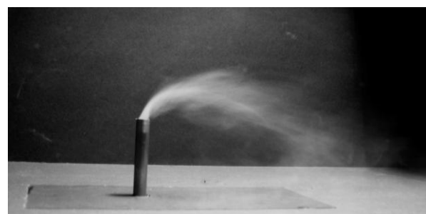
Rys. 10. Smuga emitowana w strefie cienia; u_h = 1,0 m/s ; x_s = 6H_B
